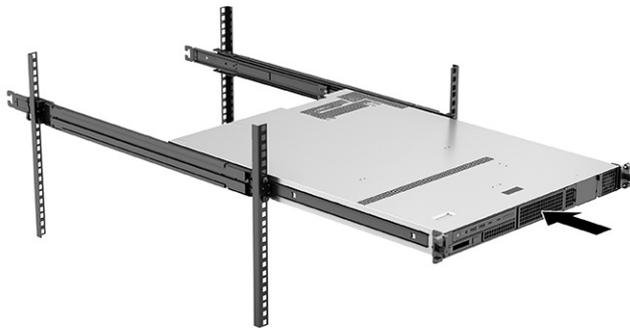
4. Secure the computer in the rack by turning the rack pull screws clockwise until tight.
