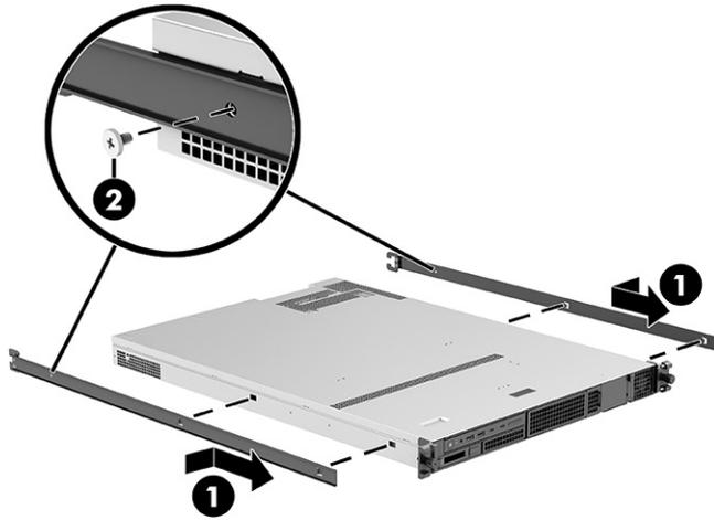
3. Slide the computer into the rack, being sure to place the glides into the rails.
