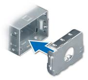
Figure 99. Installing a power supply unit blank
