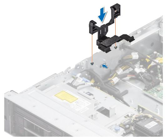
Figure 31. Installing the side wall bracket
