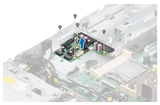
Figure 102. Removing the power interposer board
