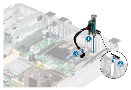
Figure 35. Installing the Serial COM port
