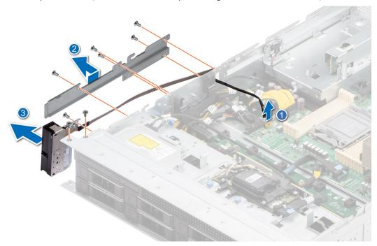
Figure 109. Removing the left control panel
