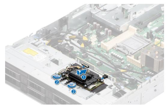
Figure 87. Installing the front mounting front PERC module
