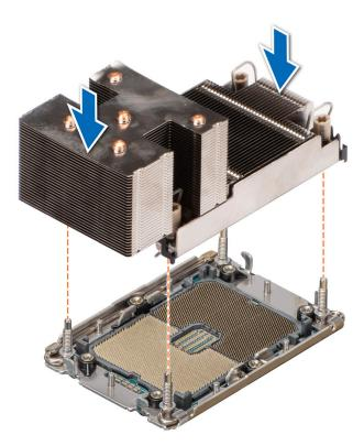
Figure 65. Installing the processor heat sink module
