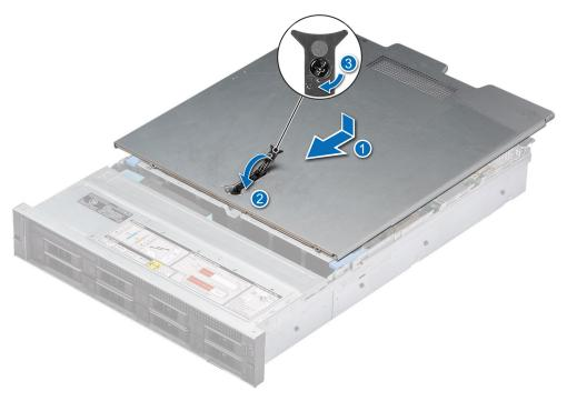
Figure 21. Installing the system cover
