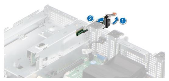
Figure 74. Removing the BOSS S2 card carrier
