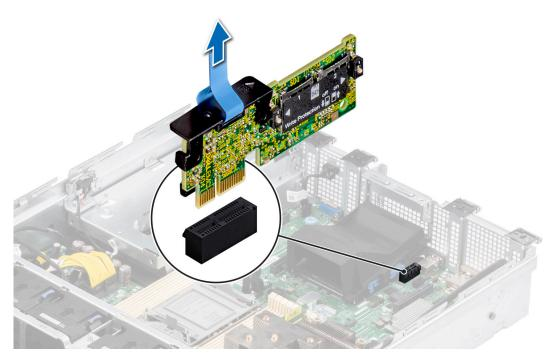
Figure 72. Removing the IDSDM module
