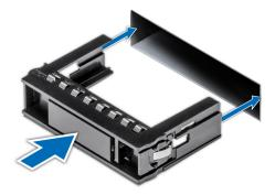
Figure 37. Installing a drive blank
