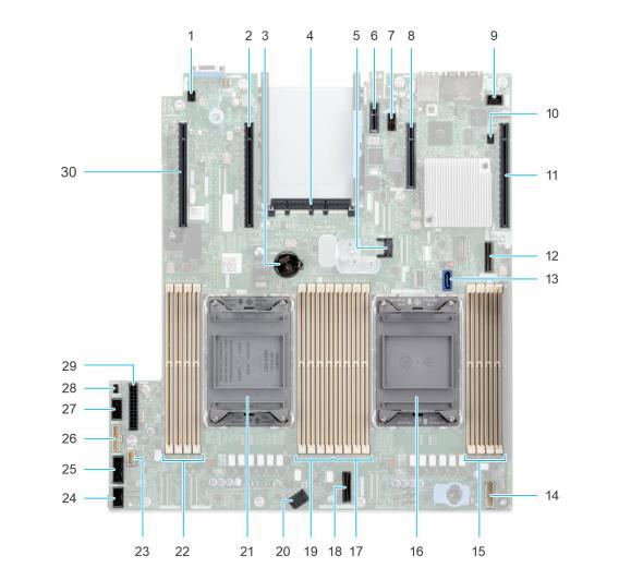
Figure 115. System board jumpers and connectors
