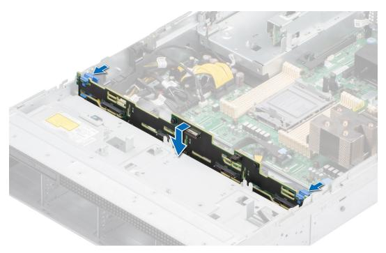
Figure 46. Installing the drive backplane
