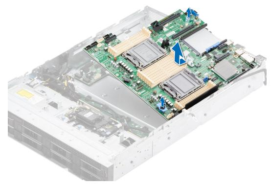
Figure 106. Removing the system board
