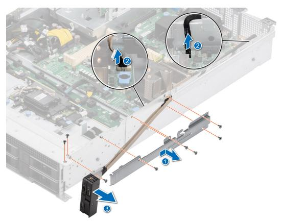
Figure 111. Removing the right control panel
