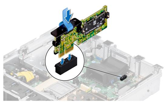
Figure 73. Installing the IDSDM module
