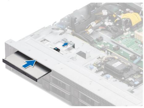
Figure 114. Installing the ODD
