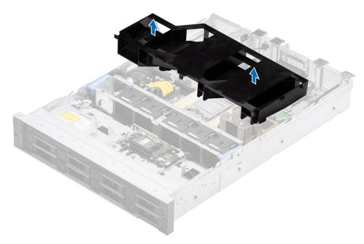
Figure 24. Removing the air shroud
