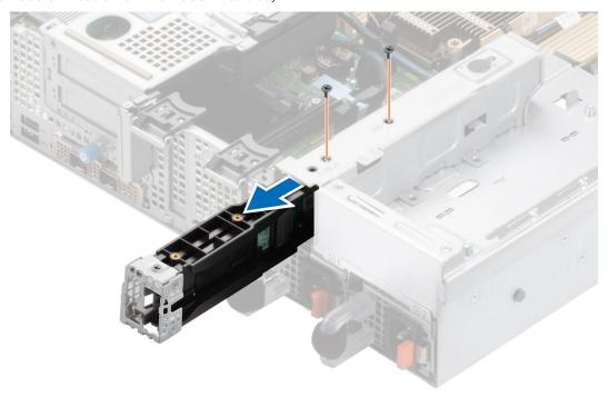
Figure 77. Removing the BOSS S2 module
