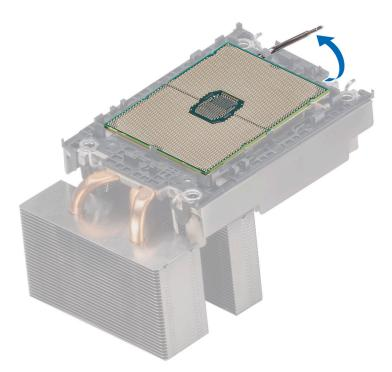
Figure 57. Lift up the TIM break lever
