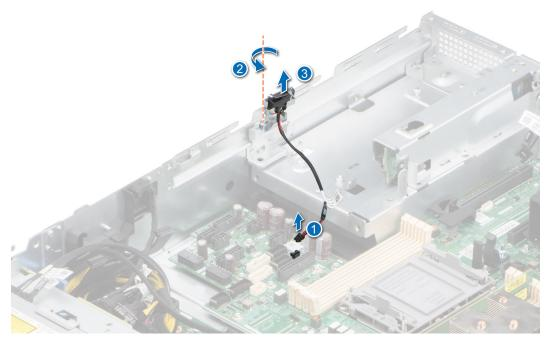
Figure 32. Removing the intrusion switch module
