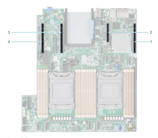
Figure 67. Expansion card slot connectors
