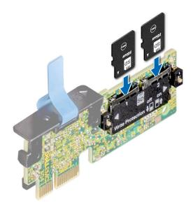
Figure 97. Installing the MicroSD card
