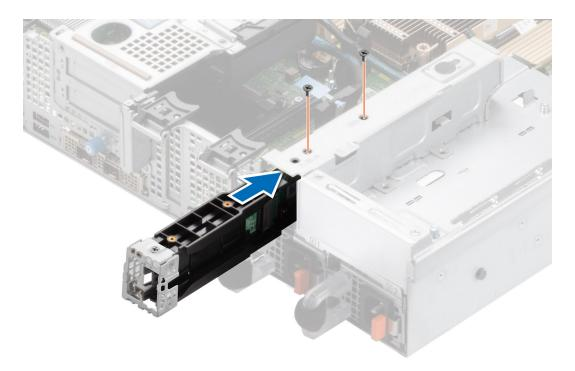
Figure 82. Installing the BOSS S2 module
