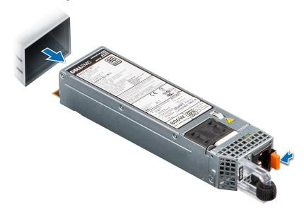
Figure 100. Removing a power supply unit
