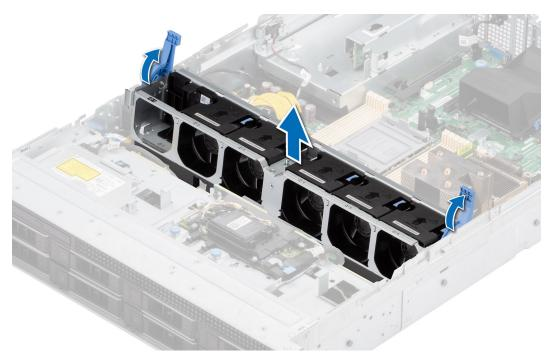
Figure 26. Removing the cooling fan cage assembly
