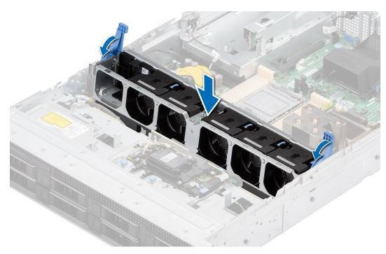
Figure 27. Installing the cooling fan cage assembly
