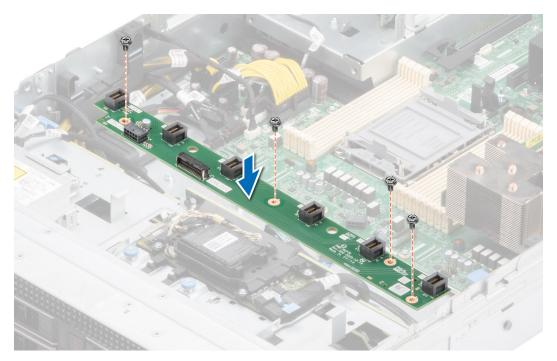
Figure 105. Installing the cooling fan cage board
