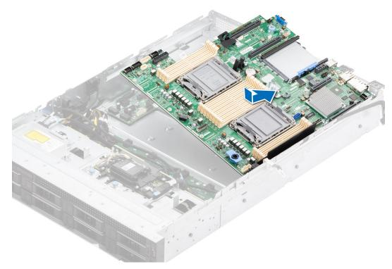
Figure 107. Installing the system board
