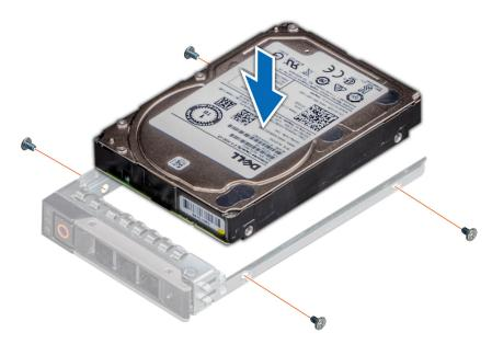
Figure 41. Installing a drive into the drive carrier
