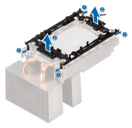
Figure 59. Removing the retaining clip
