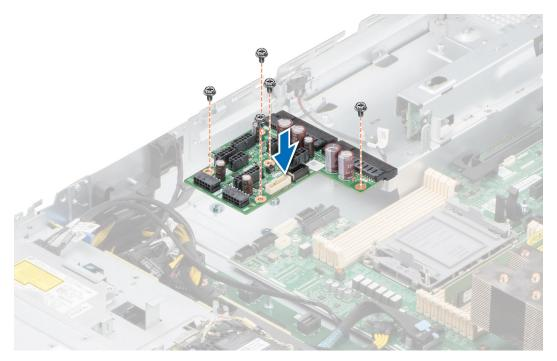
Figure 103. Installing the power interposer board
