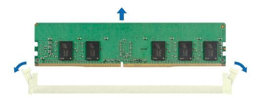
Figure 53. Removing a memory module
