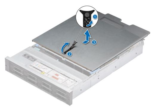
Figure 20. Removing the system cover
