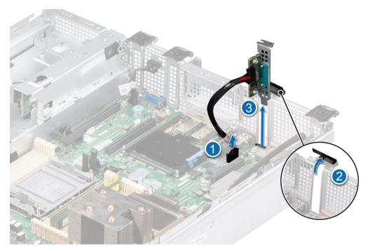
Figure 34. Removing the Serial COM port
