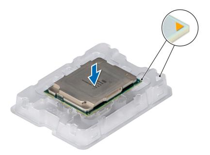
Figure 58. Aligning pin 1 marks of processor with tray
