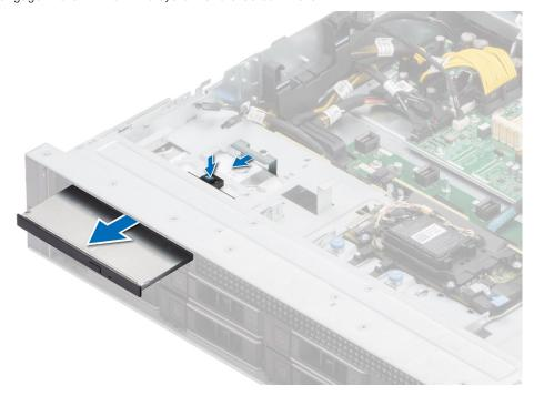
Figure 113. Removing the ODD
