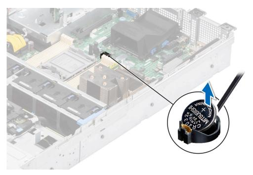
Figure 92. Removing the system battery
