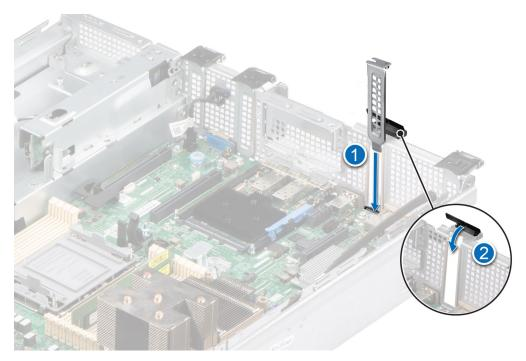
Figure 69. Installing the filler bracket
