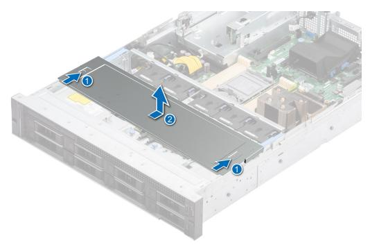
Figure 22. Removing the drive backplane cover
