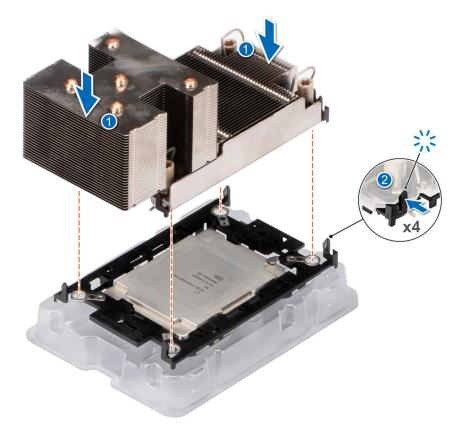
Figure 64. Installing the heat sink onto the processor
