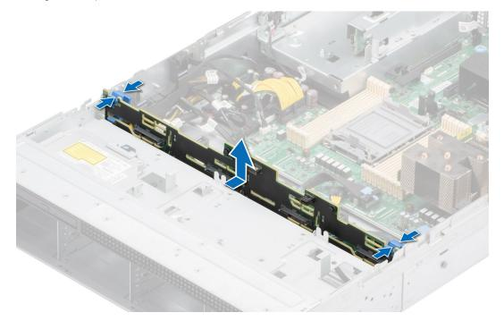
Figure 45. Removing the drive backplane
