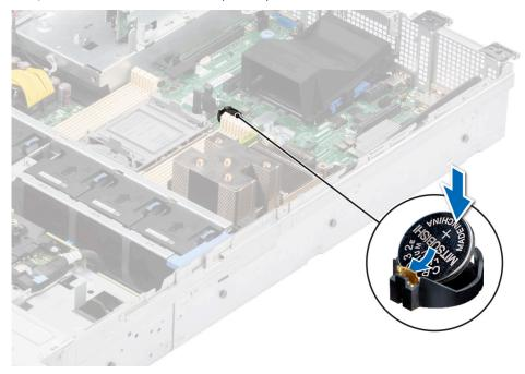
Figure 93. Installing the system battery
