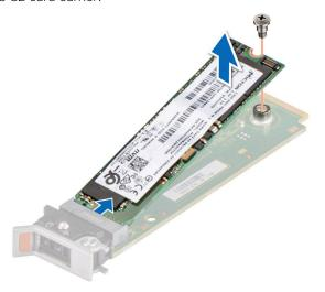
Figure 75. Removing the M.2 SSD
