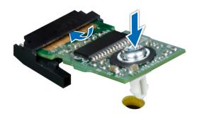
Figure 108. Installing the TPM
