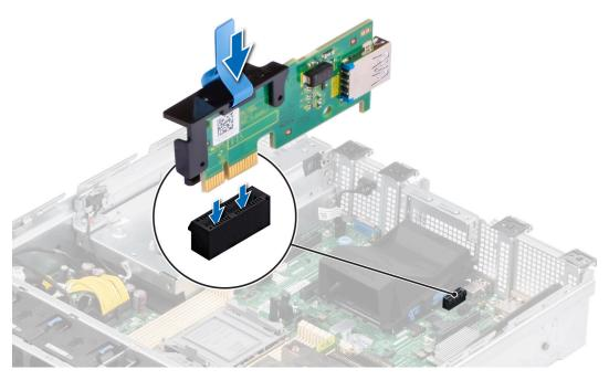
Figure 95. Installing the internal USB card
