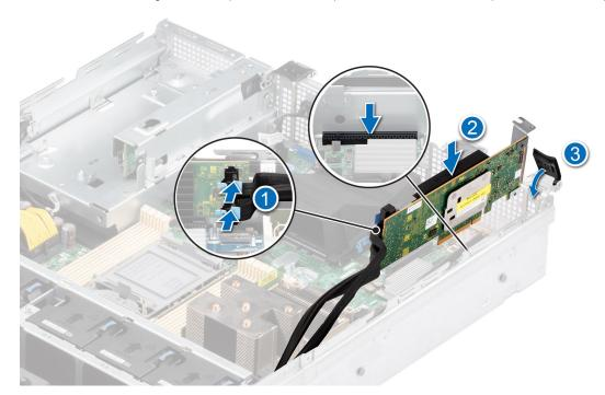
Figure 71. Installing the expansion card
