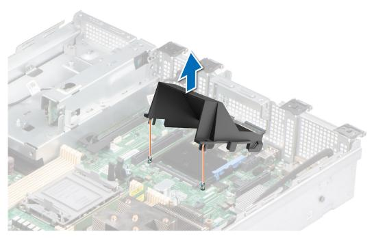
Figure 88. Removing the OCP shroud
