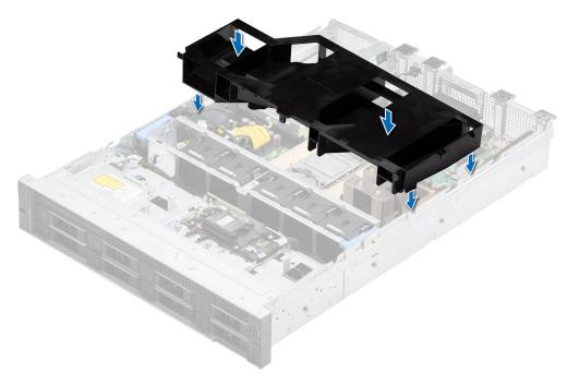
Figure 25. Installing the air shroud
