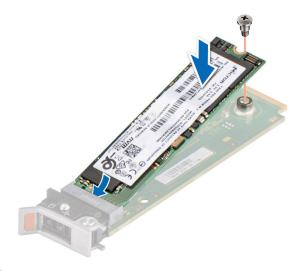
Figure 84. Installing the M.2 SSD
