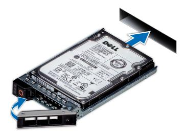
Figure 39. Installing a drive carrier
