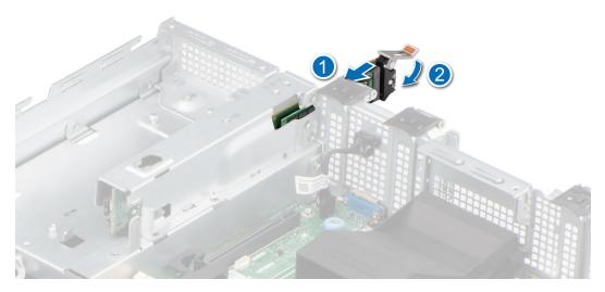
Figure 85. Installing the BOSS S2 card carrier
