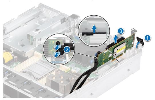
Figure 68. Removing the expansion card
