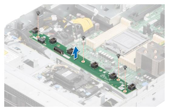
Figure 104. Removing the cooling fan cage board.
