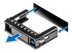
Figure 36. Removing a drive blank
