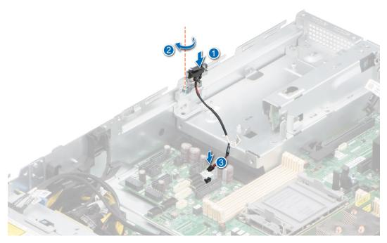
Figure 33. Installing the intrusion switch
