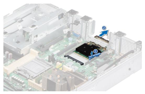
Figure 90. Removing the OCP card
