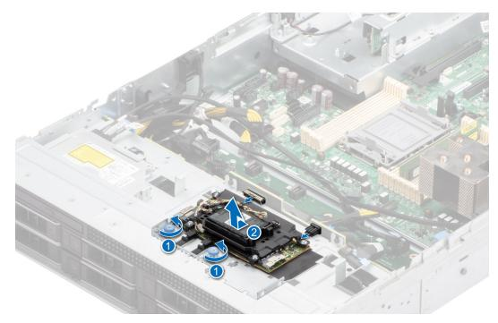
Figure 86. Removing the front mounting front PERC module
