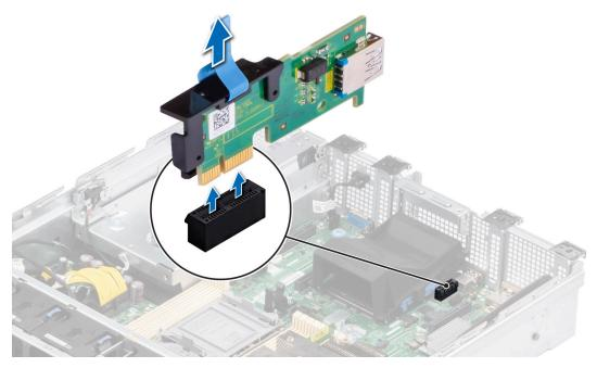
Figure 94. Removing the internal USB card
