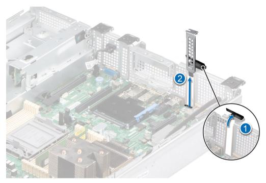
Figure 70. Removing the filler bracket
