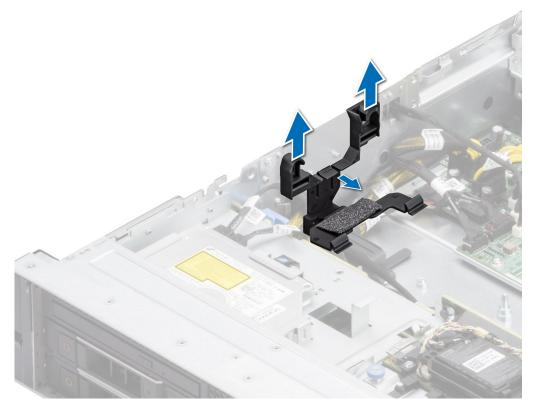
Figure 30. Removing the side wall bracket
