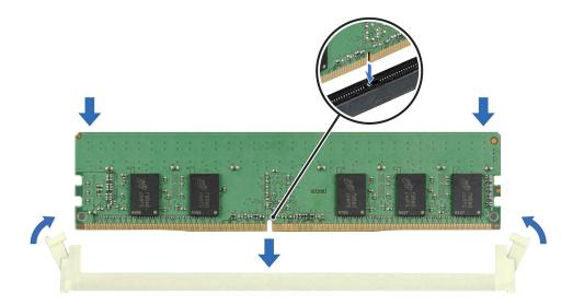
Figure 54. Installing a memory module
