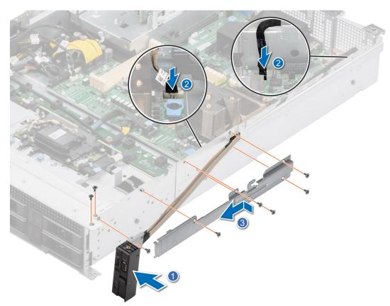
Figure 112. Installing the right control panel
