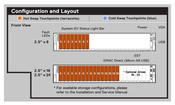
Figure 14. Configuration and layout
