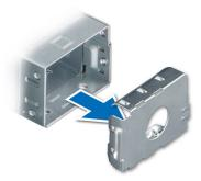
Figure 98. Removing a power supply unit blank
